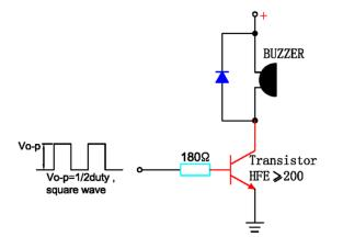
The base current lb should be high enough so that it saturates the collector current of the transistor with the CB Load
